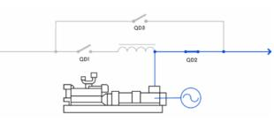
Independent Mode *mtu* Kinetic PowerPack provides energy as secondary power source, without interruption
