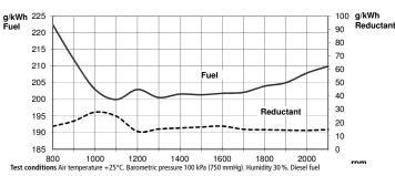
acc. to ECE R 24 Annex 6. Density of fuel 0.840 kg/dm<sup>3</sup>. Viscosity of fuel 3.0 cSt at 40°C. Energy value 42700 kJ/kg. Power test code ISO 3046. Power and fuel values +/-3%.
