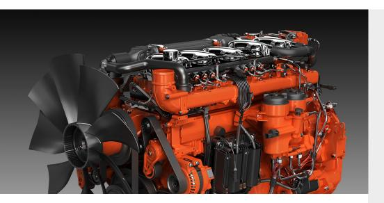
The industrial engines from Scania are based on a robust design with a strength optimised cylinder block containing wet cylinder liners that can easiliy be exchanged. Individual cylinder heads with 4 valves per cylinder promotes repairability and fuel economy.
