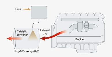
The principle for Scania SCR system
