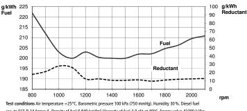
test condutions air temperature +25°C. Barometric pressure 100 kra (750 mining), humaing 30 %. Diesei tuer acc. to ECE R 24 Annex 6. Density of fuel 0.840 kg/dm<sup>3</sup>. Viscosity of fuel 3.0 cSt at 40°C. Energy value 42700 kJ/kg. **Power test code** ISO 3046. Power and fuel values +/-3%.
