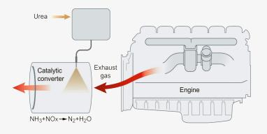
The principle for Scania SCR system
