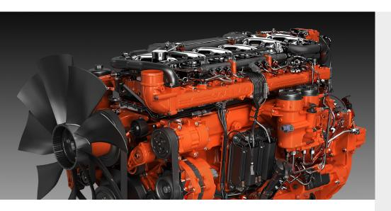
The industrial engines from Scania are based on a robust design with a strength optimised cylinder block containing wet cylinder liners that can easily be exchanged. Individual cylinder heads with 4 valves per cylinder promotes repairability and fuel economy.
