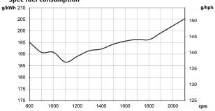
Test conditions Air temperature +25°C. Barometric pressure 100 kPa (750 mmHg). Humidity 30 %. Diesel fuel acc. to ECE R 24 Annex 6. Density of fuel 0.840 kg/dm³. Viscosity of fuel 3.0 cSt at 40°C. Energy value 42700 kJ/kg. Power test code ISO 3046. Power and fuel values +/-3%.
