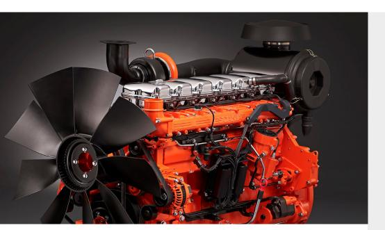
The industrial engines from Scania are based on a robust design with a strength optimised cylinder block containing wet cylinder liners that can easily be exchanged. Individual cylinder heads with 4 valves per cylinder promotes reparability and fuel economy.
