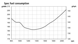
Test conditions Air temperature +25°C. Barometric pressure 100 kPa (750 mmHg). Humidity 30 %. Diesel fuel acc. to ECE R 24 Annex 6. Density of fuel 0.840 kg/dm³. Viscosity of fuel 3.0 cSt at 40°C. Energy value 42700 kJ/kg. Power test code ISO 3046. Power and fuel values +/-3%.
