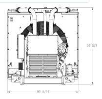
Drawing above for illustration purposes only, based on standard open power 480 volt generator set. Lengths may vary with other voltages. Do not use for installation design. See website for unit specific template drawings.
